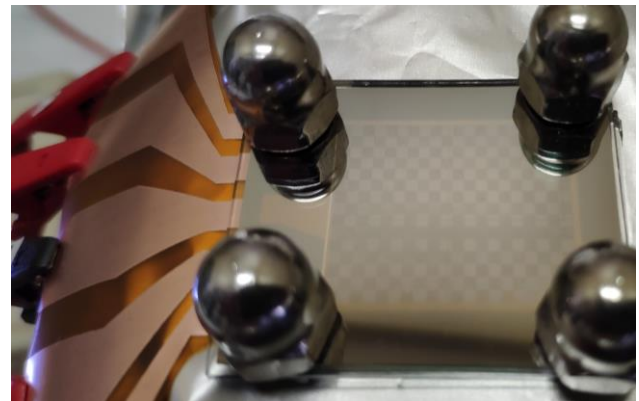
Figure 5. Active matrix MEMS shutter demonstrator testing on a hotplate.
