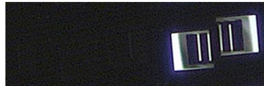
Figure 4. Microphoto of bottom view of the optimized illuminated shutters (left: collapsed shutter, right: released shutter).
